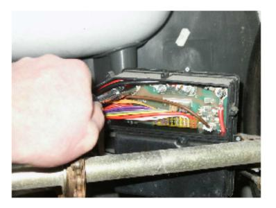
You need to also disconnect the brown +12v connector attached to X5 (shown disconnected here)
