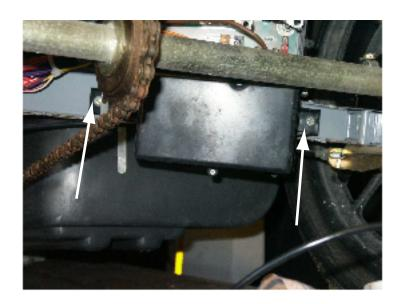
To remove the control box undo these two marked bolts. When removed the control box will slide to the right slightly to allow it to slip out of the retaining large cable tie.
