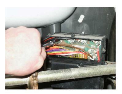
You need to also disconnect the brown +12v connector attached to X5 (shown disconnected here)
