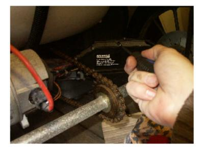
Undo retaining screws and remove control box cover.
