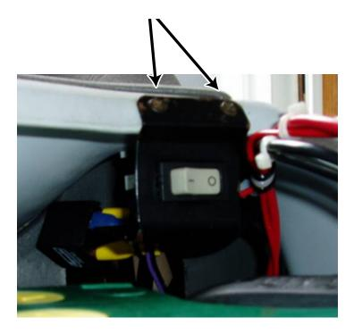
Undo the two screws that hold the lights on/off switch in place.
