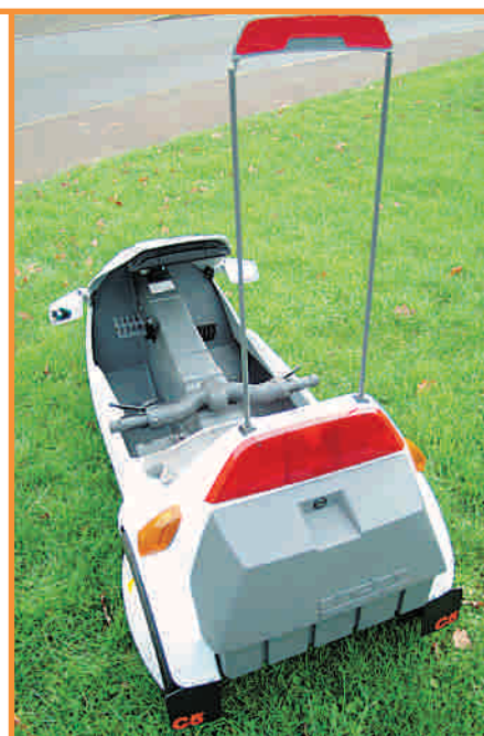
An official Sinclair accessory – the 'High-Vis Mast' is simply a reflector on poles which fits into two pre-moulded slots.
