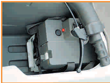
Left: The battery cover comprises a key-operated 'master security' switch and a cut-out button.
