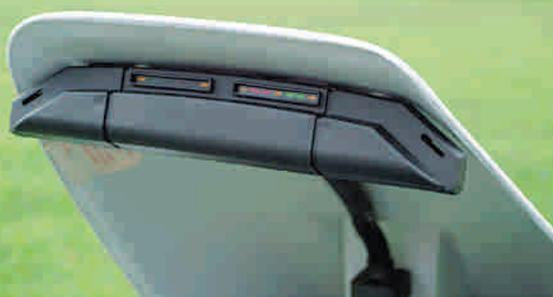
The C5's instrument pod comprises two LED bar graphs to show the motor load (left-hand side), and battery level (right-hand side).
