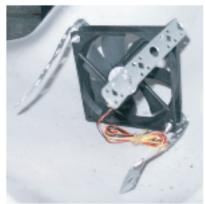
Fit 3 or 4 of the brackets to the motor in the fashion shown here. We found that 3 worked perfectly well and was easier to fit - but 4 have been supplied.
