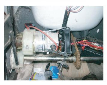
Finally - simply tighten the jubilee clip until the tangs are held firm and check that the fan mounting screws are also tight
