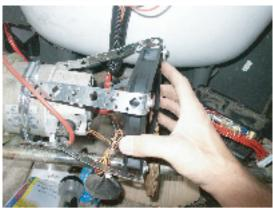
Next - wrap the jubilee clip around the motor circumference and attach until there is just a few millimeters slack all round.
